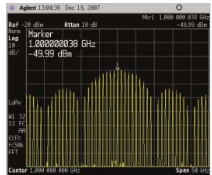
Figure 12. Same signal as figure 11 with span decreased to 5 kHz and bandwidth decreased to 100 Hz.
